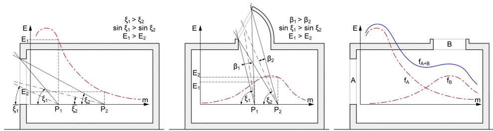
Illumination distribution caused by side-lights, skylights and combined daylighting systems
